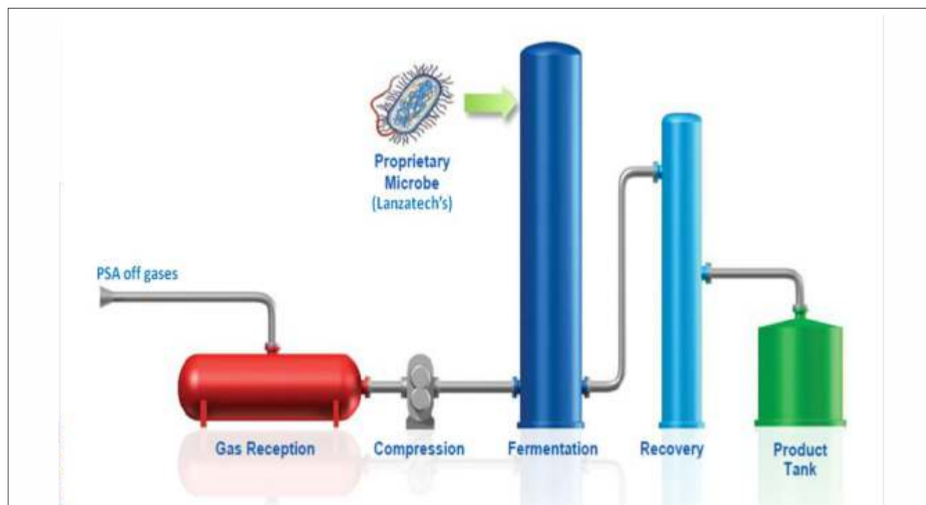
Schematic of ethanol production from HGU PSA off gas using gas fermentation process
